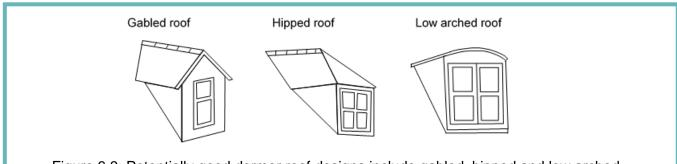
Figure 6.3: Potentially good dormer roof designs include gabled, hipped and low arched roofs.
