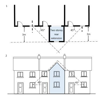
Figure 4.3: The 45 Degree Rule illustrated on a two-storey extension for a terraced property.
