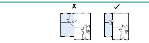
Figure 5.2: Side extensions should be no more than half the width of the original house to ensure subservience and visually pleasing proportions.
