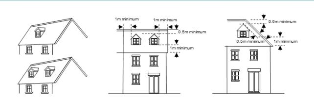
Figure 6.1: The three diagrams illustrate the advised positioning of dormers:
