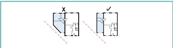
Figure 5.3: Side walls of extensions should remain parallel with the original house.
