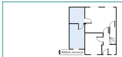
Figure 5.1: Side extensions should be set back at least 900mm from the front main wall of the house to ensure subservience.
