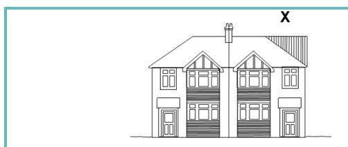
Figure 7.1: The hip to gable extension here results in a negative imbalance to the symmetry of the pair of semi-detached dwellings.
