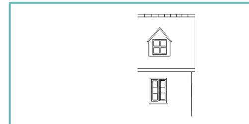
Figure 6.2: The dormer's size allows the main roof to remain the dominant feature, and the dormer window is smaller than the window on the floor below.
